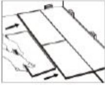
Full loose plank and use the long side to tap against the prior row to ensure no gapping.
